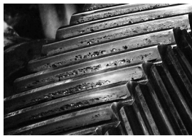
Figura 2 Pitting corrosion.
