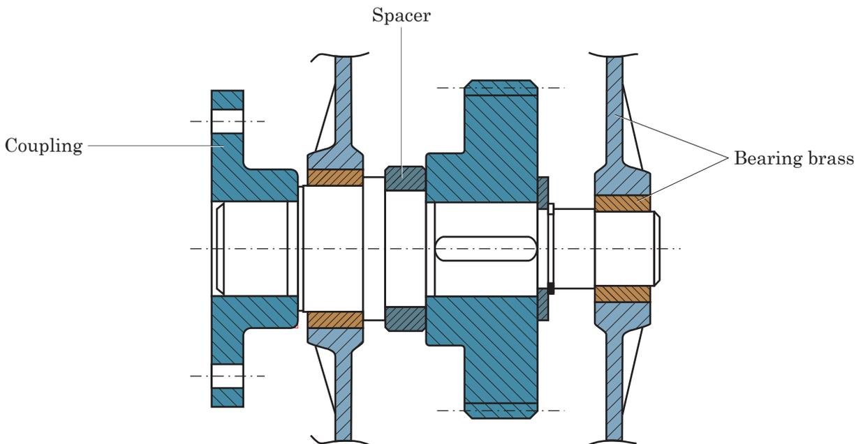
Fig. 44.1 - Some elements of a shaft. The shaft can transmit torque to another shaft by means of coupling.
