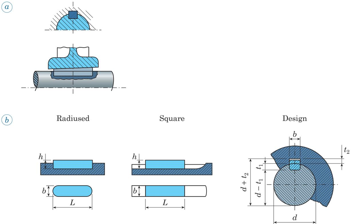
Fig. 44.4 - a) The tapered key (1:100) when assembled into keyseat prevents any relative motion between shaft and hub.
