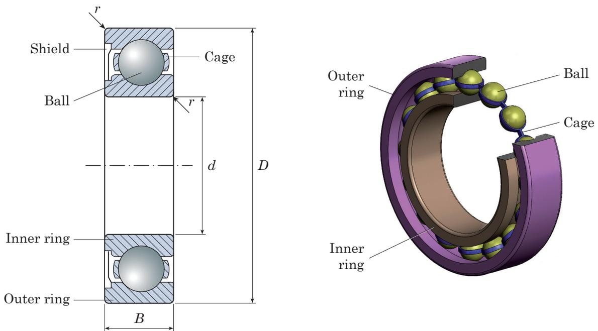
Fig. 44.13-b - Nomenclature of a ball bearing.
