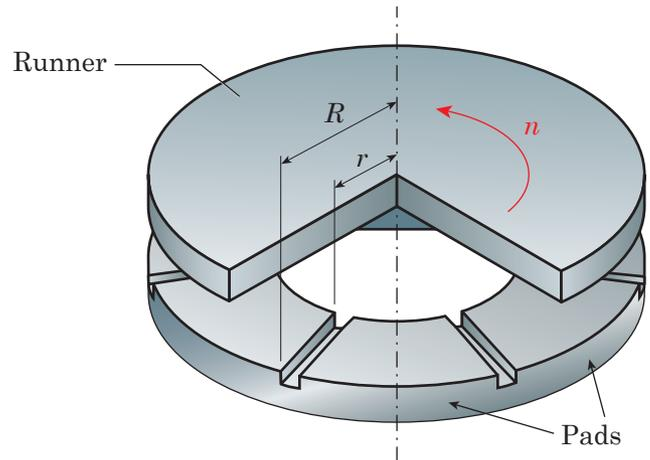
Fig. 44.11-a - Fixed-pad thrust bearing.
