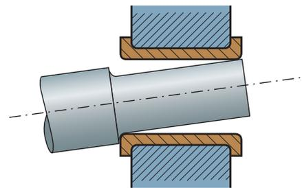
Fig. 44.3-b - Too large deflection of a journal in respect of the bearing.
