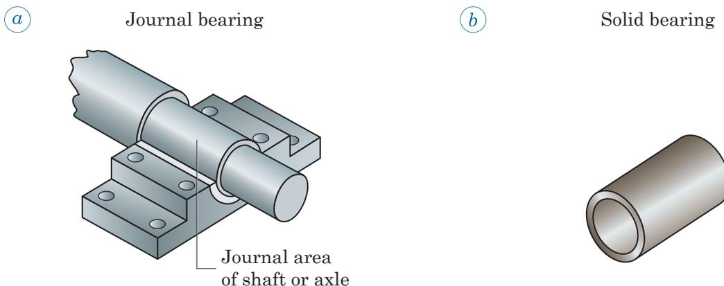
Fig. 44.5 - Journal bearing (a) and solid bearing (b).
