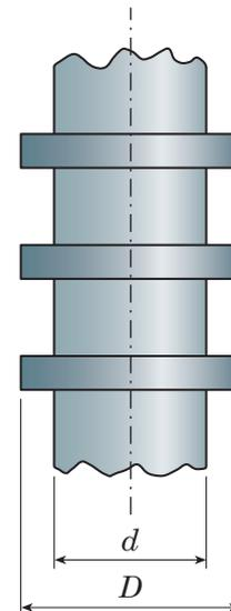
Fig. 44.11-b - Intermediate thrust bearing with more runners (annular collars with diameter  $D$ ) on a shaft diameter  $d$ :  $D = (1.5 \div 2.0)d$ .
