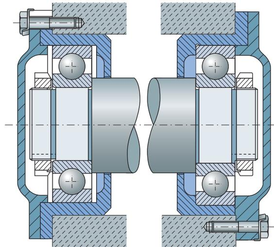
Fig. 44.14 - Mounting of radial rolling bearings: the outer ring (on the left) is not axially blocked. In a couple of rigid bearings mounted on a shaft, only one must be axially blocked, while the other one must be free to account eventual longitudinal expansion or contractions of the shaft.
