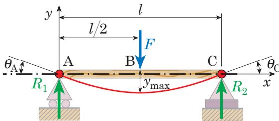
Fig. 44.3-a - Linear deflection  $y_{\max}$  and slope  $\theta$  of a deflected shaft.
