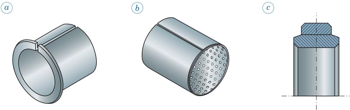
Fig. 44.8 - Various types of bushes (usually as one piece, but in two halves to make their mounting possible):
