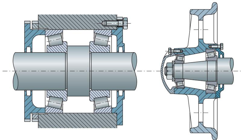
Fig. 44.15 - Angular contact cylindrical roller bearing are designed to combine radial and axial loading.
