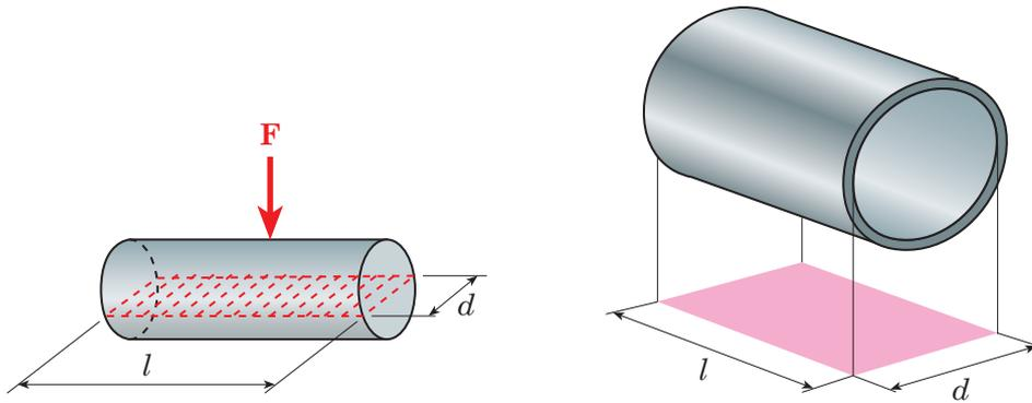
Fig. 44.9 - The projected area, interested by the average contact pressure  $p$  relative to the load  $F$ , is given by the product of journal diameter  $d$  for its length  $l$ .
