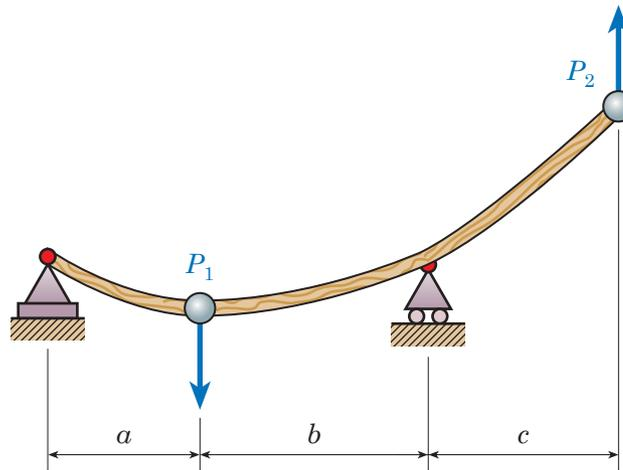
Fig. 44.17 - Shaft of *Example 44.3* with  $a = 0.4$  m,  $b = 0.6$  m and  $c = 0.5$  m.
