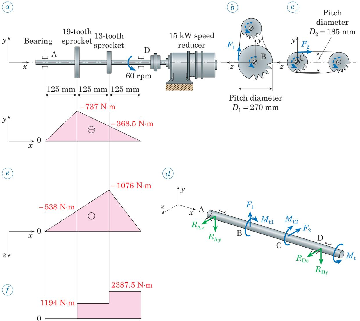
Fig. 44.2 - Bending moments and torque diagrams of a solid steel shaft driving two sprocket wheels (from *Figure 21.9*); similar sprockets and roller chains are commonly used on bicycles. Calculations aimed to shaft verification are shown in *Example 21.4*.
