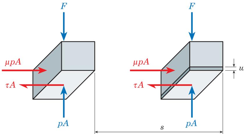
Fig. 44.10 - Sliding block moving along a plate with  $\mu$  as a friction coefficient and subjected to linear wear  $w$  during the displacement  $s$ .
